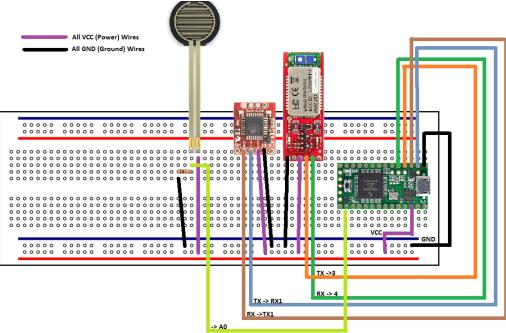
The image below is the above diagram in real life. This device currently will read in the amount of force being applied to the force sensitive resistor, and write it to an SD card. The data being read and written is simply integers.
