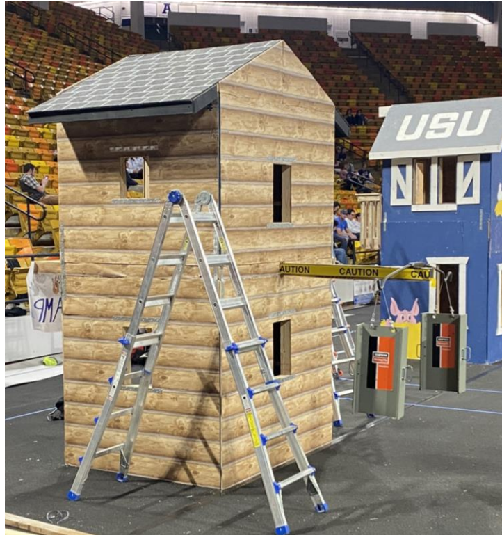
Figure 6- 7: Cantilever Deflection Test
