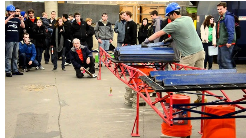
Figure 2-2: Vertical Load Test [2]
