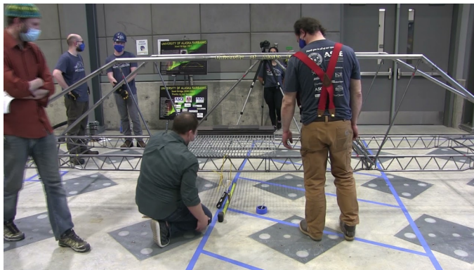
Figure 10-2: Lateral Load Test [6]
