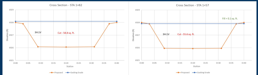
Figure 37: Upstream cross sections
