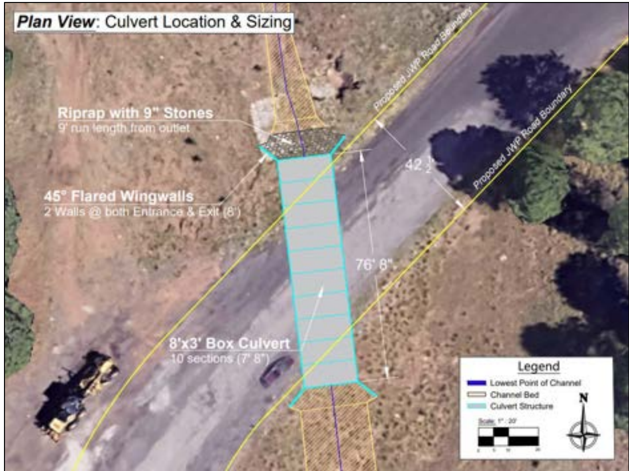
Figure 5-6: Plan view of final hydraulic structure design
