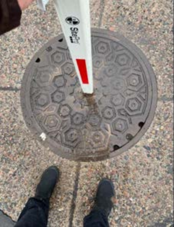
Level rod and benchmark (manhole)
