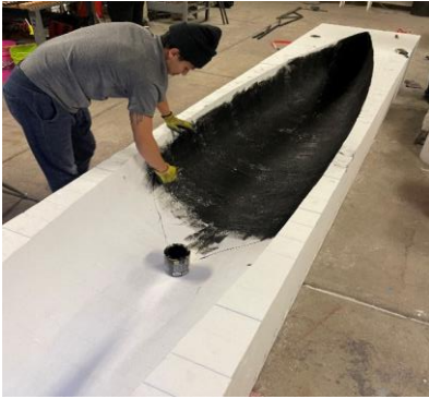
Figure 4: Application of Releasing Agent
