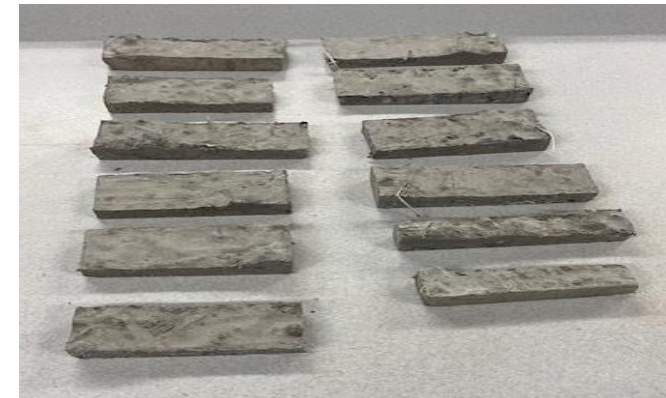
Figure 9: Flexural Testing Bricks
