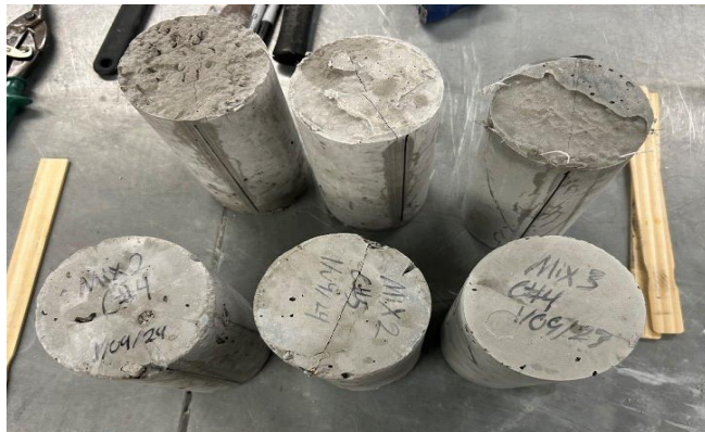
Figure 7: Concrete Testing Cylinders
