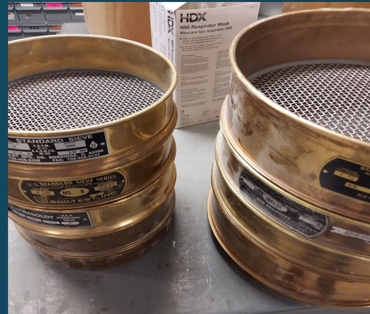
Figure 6: Stacked sieves used for a gradation & size test. -Courtesy of Jon Duran.
