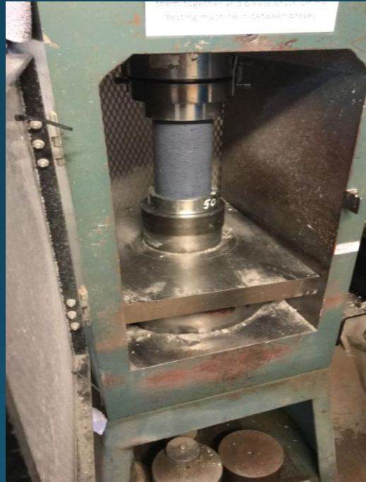
Figure 9: Concrete cylinder break. -Courtesy of Dylan Condra.
