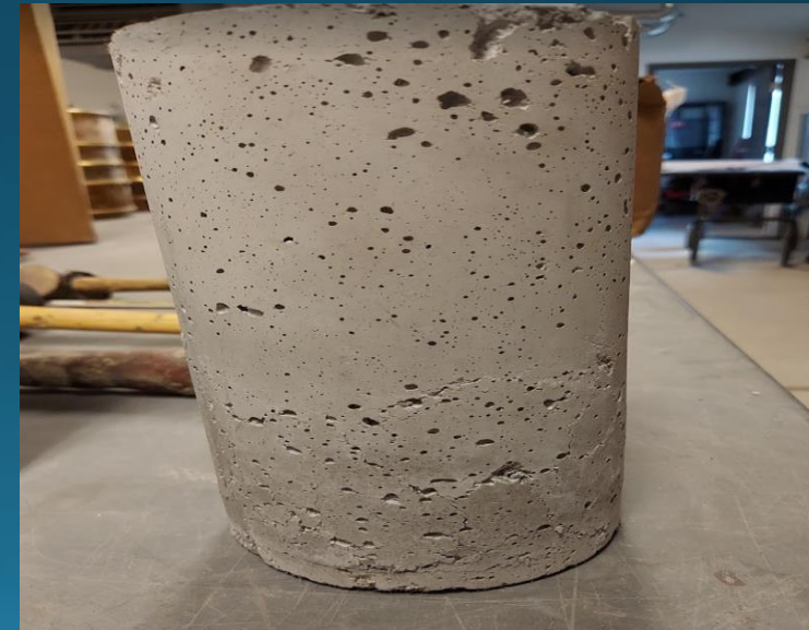
Figure 7: Concrete Cylinder for Compression Test. -Courtesy of Jon Duran.
