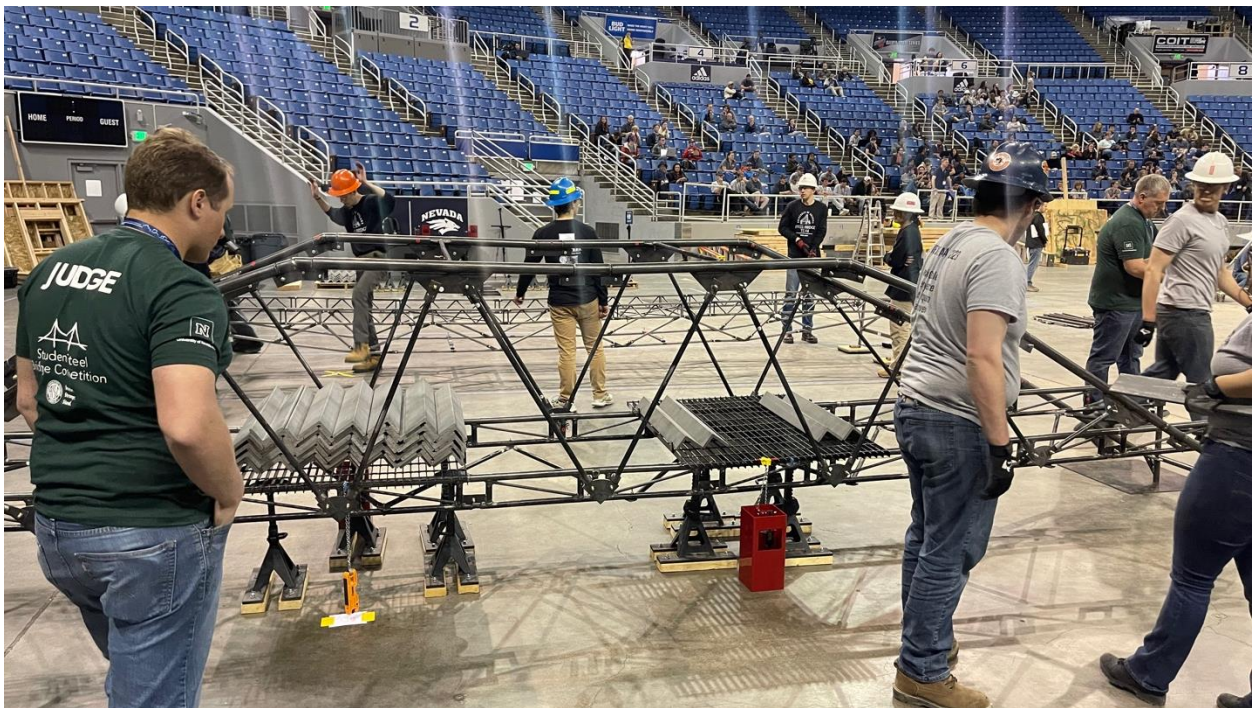
Figure 18: Twenty-five-pound Weights on Bridge
