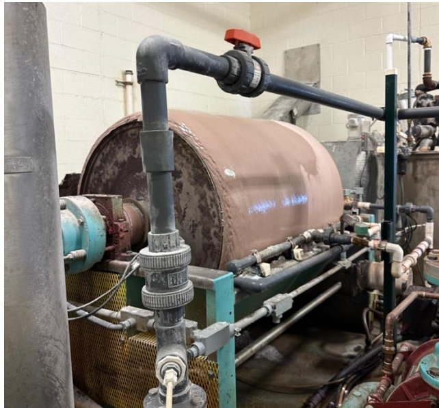
Figure 1- 3: Current rotary drum vacuum filter
