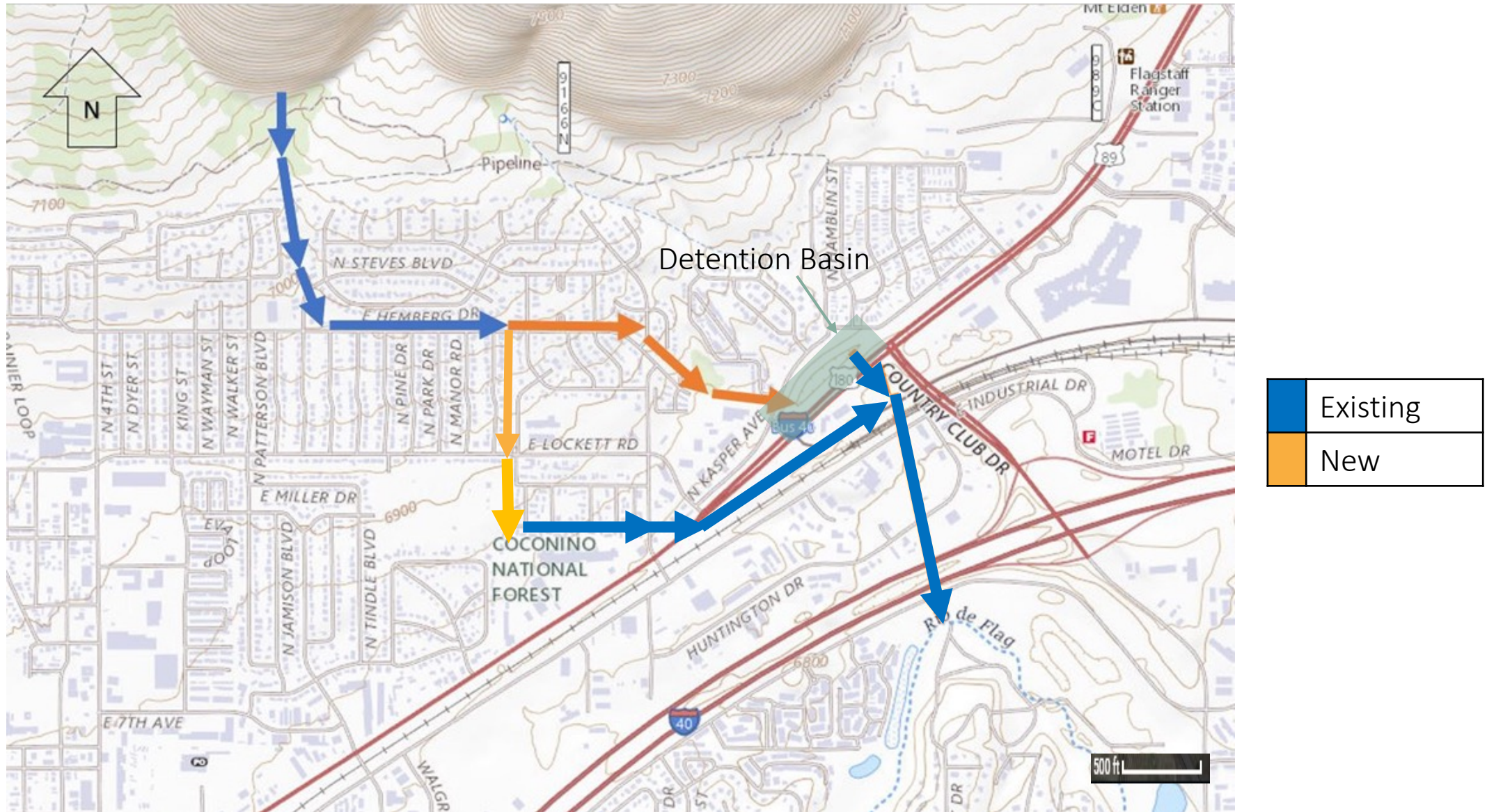
Figure 12: Drainage System and Channel Rehabilitation Credit: USGS & Caleb Smith
