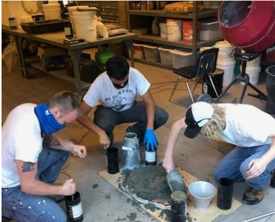
Figure 2: Mentees Conducting Slump Test [1]
