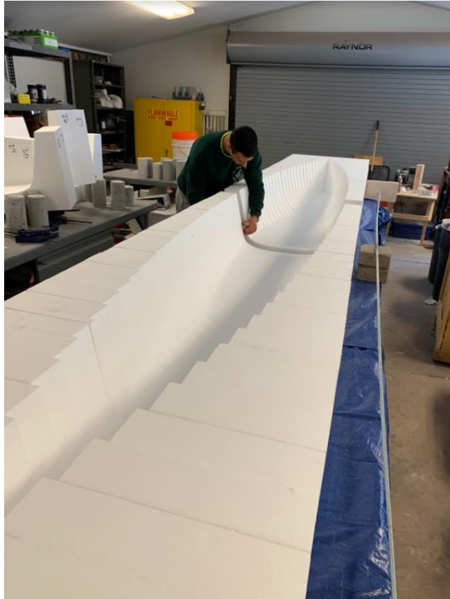
Figure 12: Gluing Mold Pieces Together Picture Credit: Steven Procaccio
