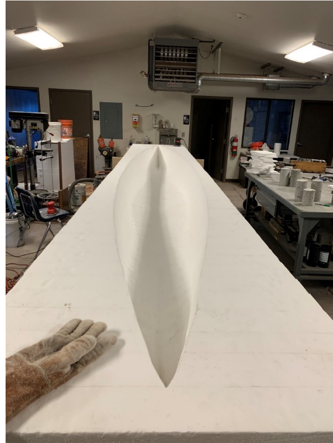
Figure 13: Mold After Sanding Picture Credit: Hunter Kassens
