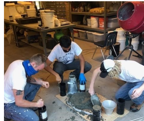
Figure 6: Ponderosa Concrete Canoe Team, 2020-2021, Mentees Performing Slump Test [5]
