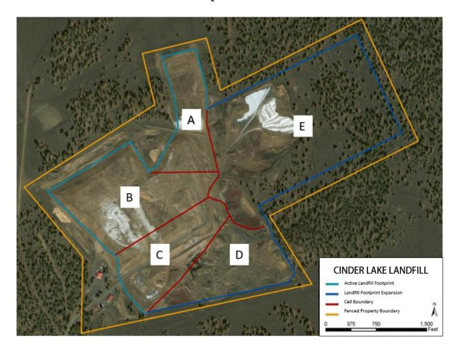
The Cinder Lake Landfill consist of 5 different cells. Currently only cells A-C are in use. Cells D and E will be used for further expansion. Only cells A-C are considered for the project, which consists of 108 acres.
