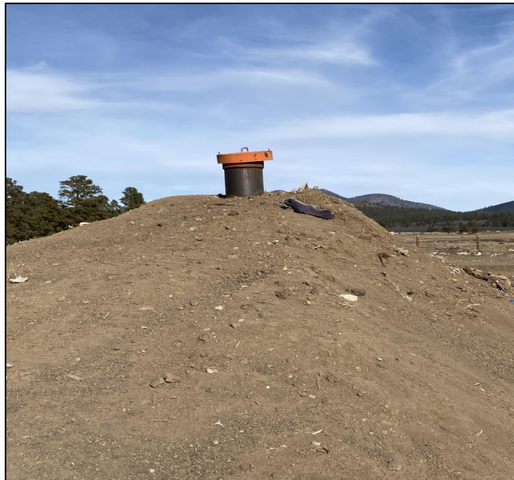
Figure 2-1: Hydroprobe Monitoring Well
