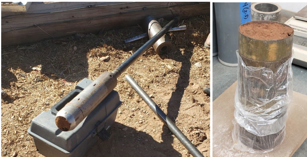
Figure 3: Collected sample in hand operated device (right) and sample in rings at lab (left).
