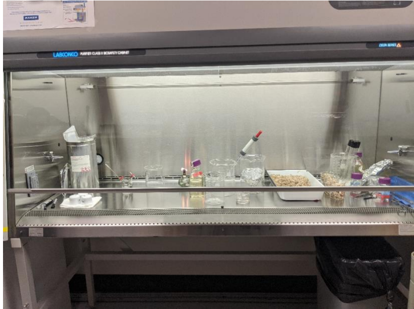
Figure 3-6: Laminar Flow Hood Setup
