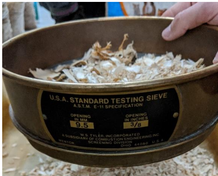
Figure 3-3: Sieve size 9.5 mm With Aspen Media
