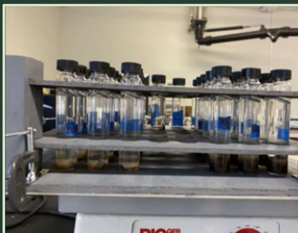
Figure 10: Sample Vials on Shaker Table
