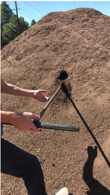
Figure B.6 Pile 2 Sampling Auger
