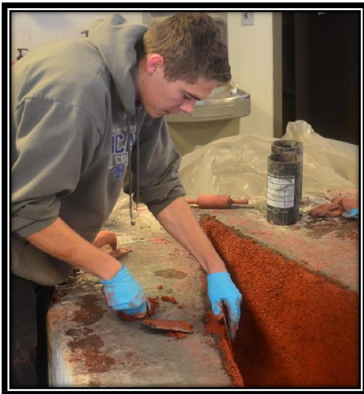
Figure 20: Quality assurance was done on the rim of the canoe by trowel and hand.
