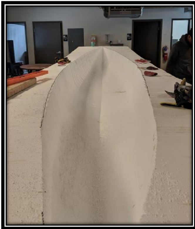
Figure 7: Once little sections were all glued, then the metal sheets and the rods come into play where bolts are used to tighten it all together. This picture shows all the cross-sections pushed together ready to be sanded.
