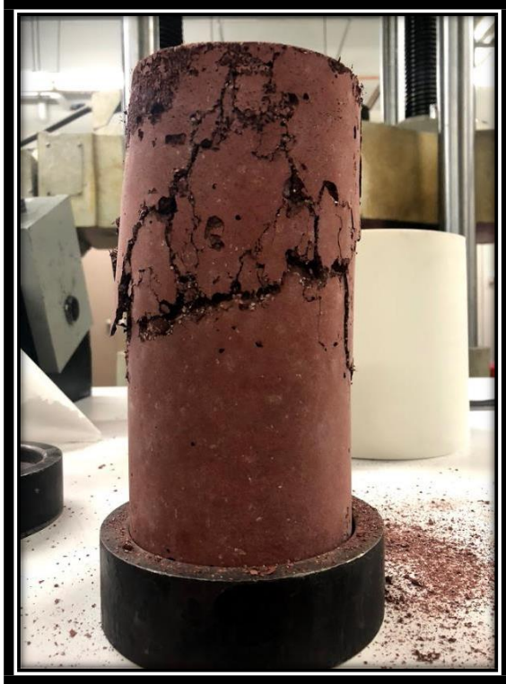
Figure 39: A compression break of the finishing mix cylinder was tested for the compressive strength of the mix.
