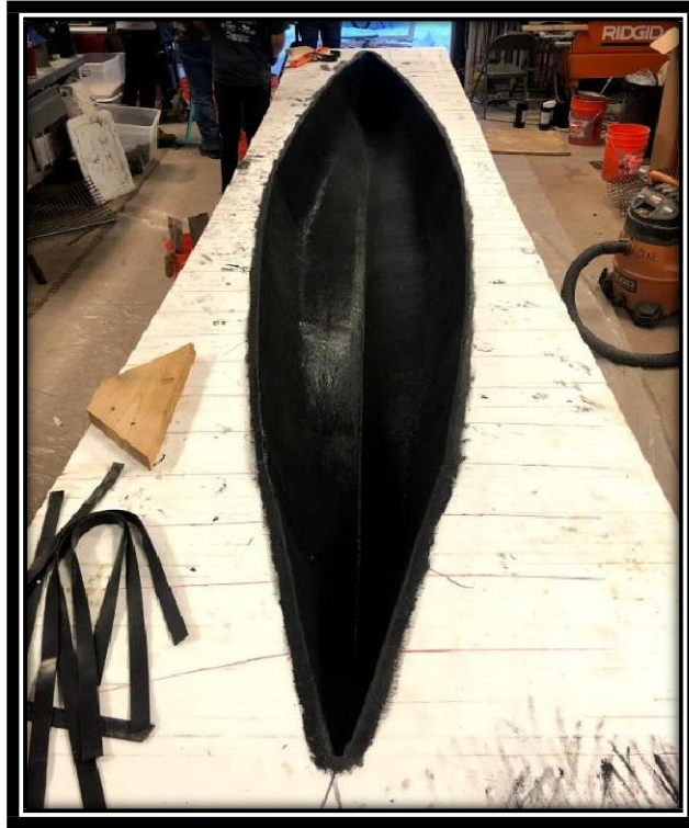
Figure 11: The flex seal is then dried for at least 24 hours before the canoe construction began.
