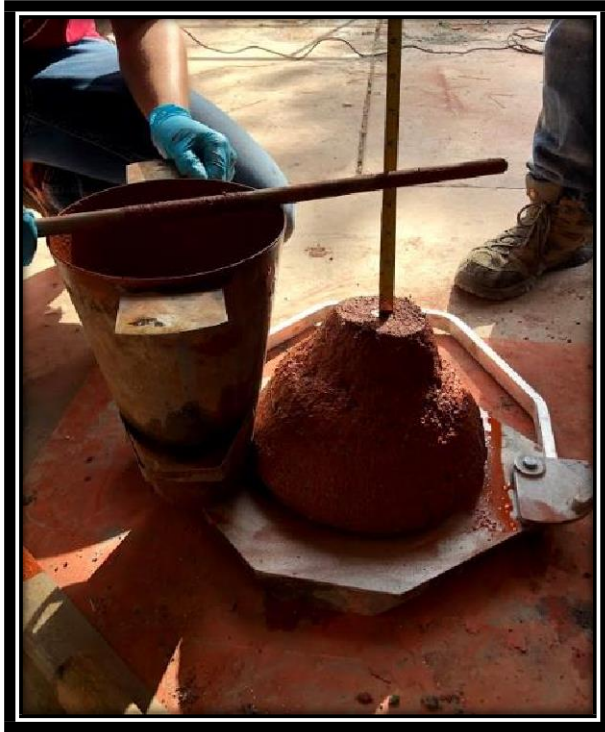
Figure 37: A slump test was conducted to analyze and test the mix.
