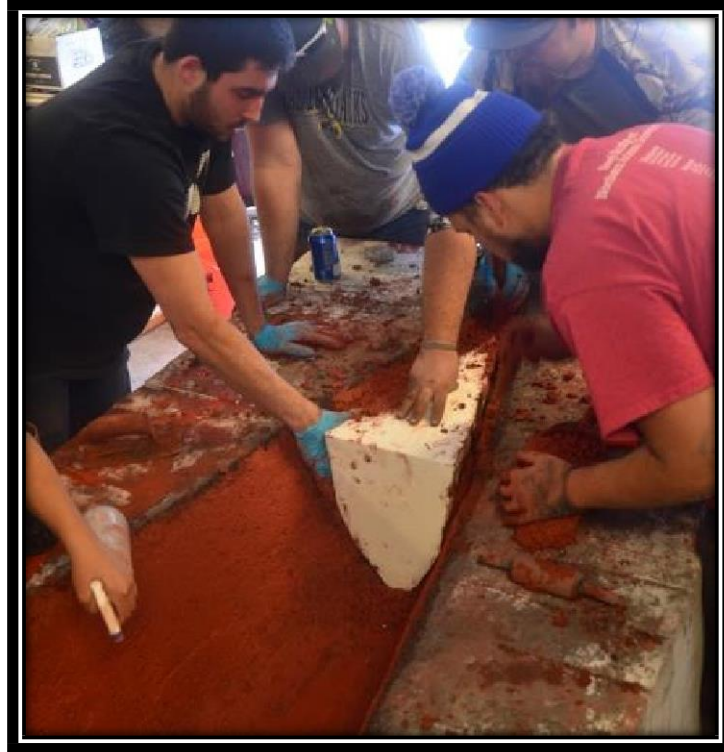
Figure 21: End caps were put in at the end of the canoe, and were then covered with the red finishing layer of concrete.
