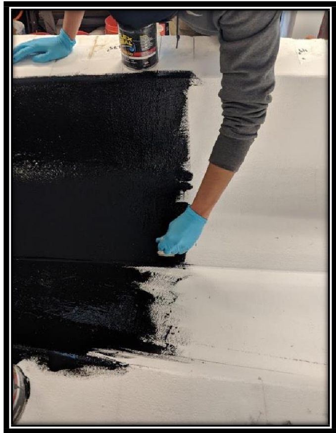
Figure 10: Once the sanding process was complete, flex seal was placed on the whole inside of the mold to help reduce the concrete from sticking. It also helps the concrete to be placed on a smooth layer.
