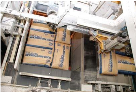
Sacking Operation, Clarkdale AZ
