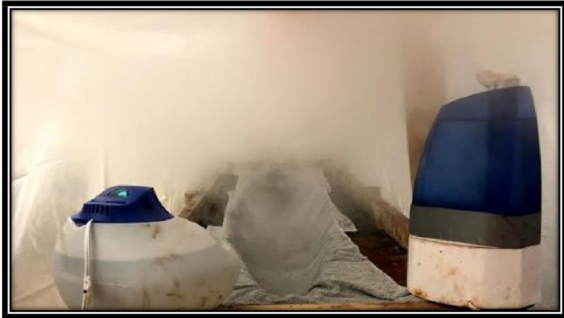
Figure 38: Four humidifiers were placed at each corner of the mold inside the curing chamber. Salt was also put into the water of the humidifiers. This was the team's way of ensuring that the canoe was properly moist and curing correctly at all times. The humidifiers were checked and refilled every 12 hours.
