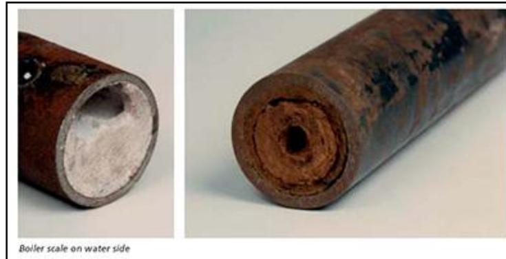
Figure 1: Scaling on pipes [2]
