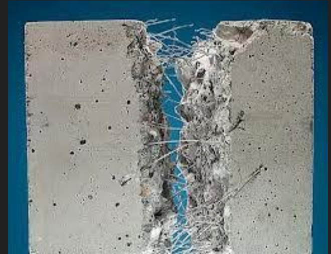
Figure 14: Concrete modular block utilizing plastic fiber reinforcement [11]
