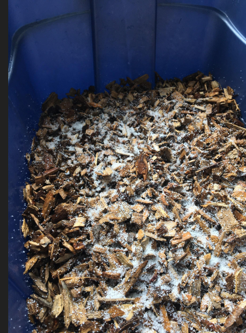
Figure 7: Wood Chips soaking in aluminum-sulphate and water solution [Photo taken by: Sam Carnes]
