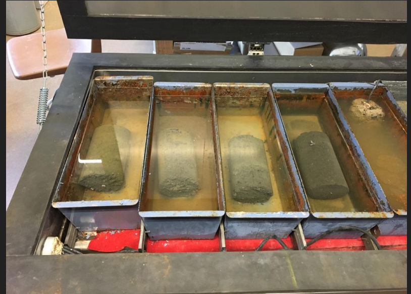
Figure 12: Freeze-Thaw Test [Photo taken by: Sam Carnes]
