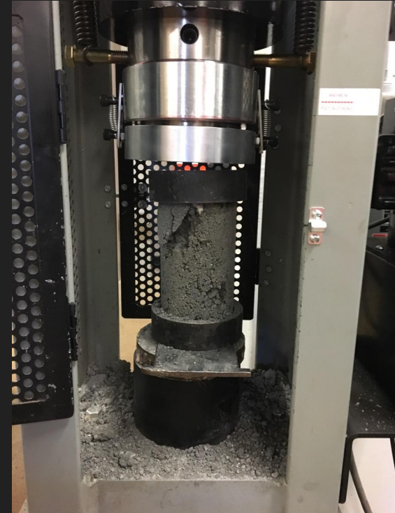
Figure 10: Compressive Strength Test [Photo taken by: Teo Albers]
