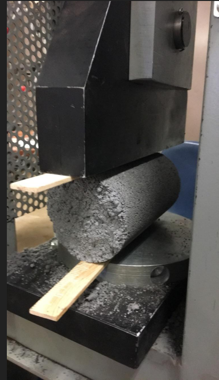
Figure 11: Tensile Strength Test [Photo taken by: Teo Albers]
