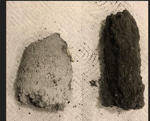
Figure 14: Freeze-Thaw Test failed specimen [Photo taken by Teo Albers]
