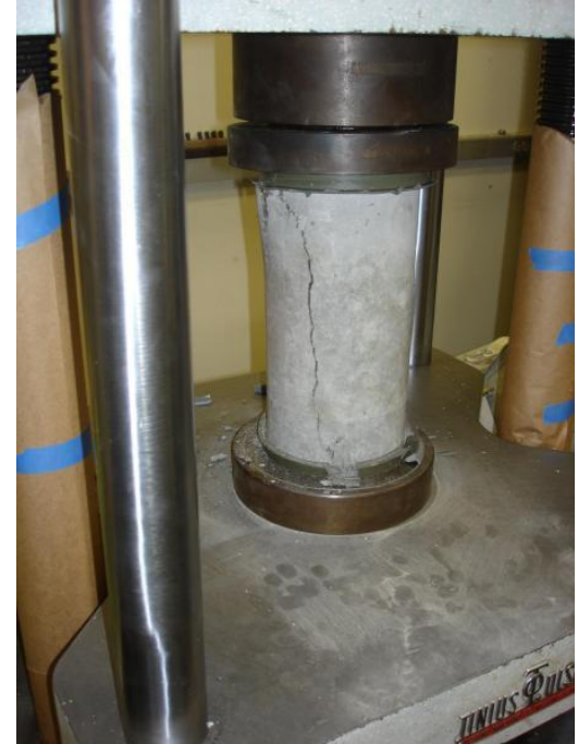
Figure 11: Compressive Strength Test [13]
