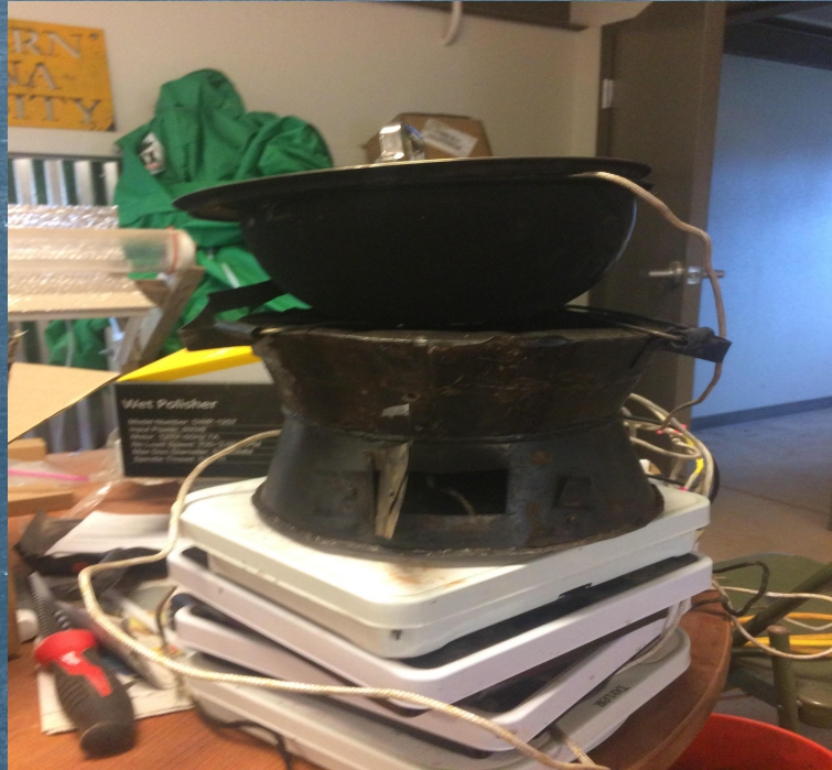
Figure 9: Thermocouple Jiko Stove Set-up (photo by: Xiaoying Tang)
