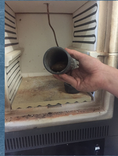
Figure 6: Briquette Chamber in Pyrolysis Oven (Photo by: Mohammad Alkandari)
