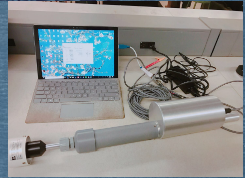
Figure 7: Particulate Profiler (photo by: Xiaoying Tang)
