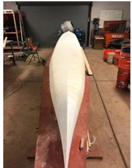
**Figure 8: Completed Mold**
