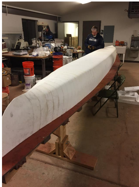
Photo 8. Organized Mold Cross-Sections: The mold was organized and laid out on the construction table to prepare for saran wrapping.
