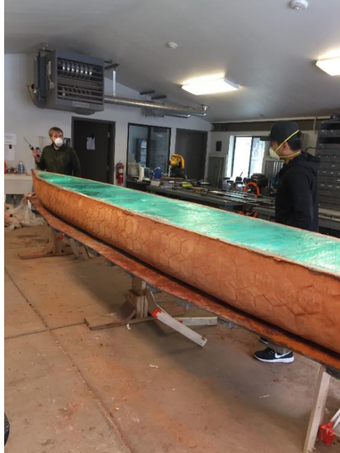
Photo 3. Preparing for Mold Removal: The curing chamber was taken down and the canoe was flipped to prepare the removal of the styrofoam mold.
