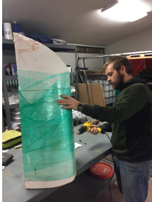
Photo 9. Applying Saran Wrap: Saran wrap was added to the mold to ensure that concrete would not stick to the mold during casting. A heat gun was used to allow the wrap to shrink and tighten around the mold.
