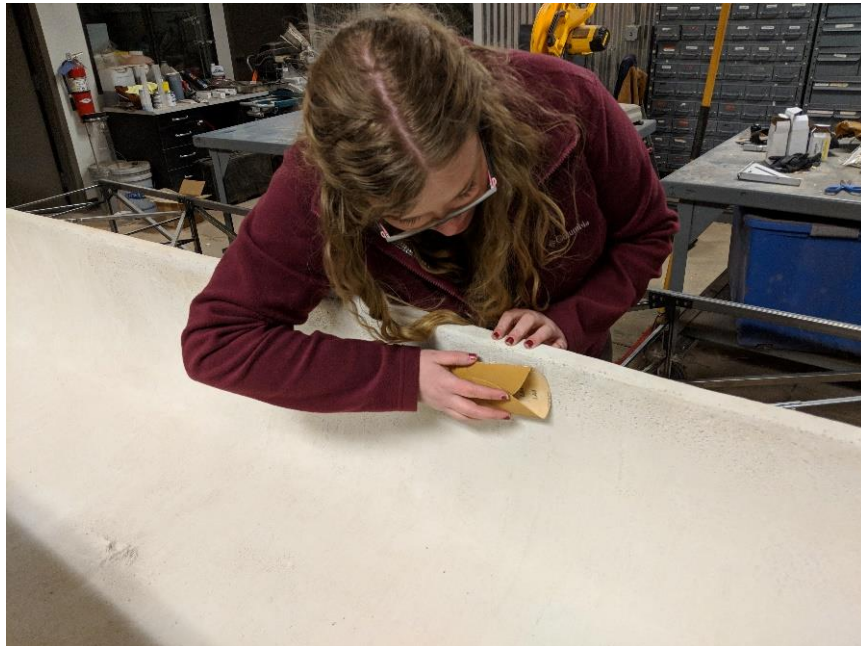
Photo 5. Incasing the Bow/Stern: The floatation in the bow and stern was encased in structural mix #1.
