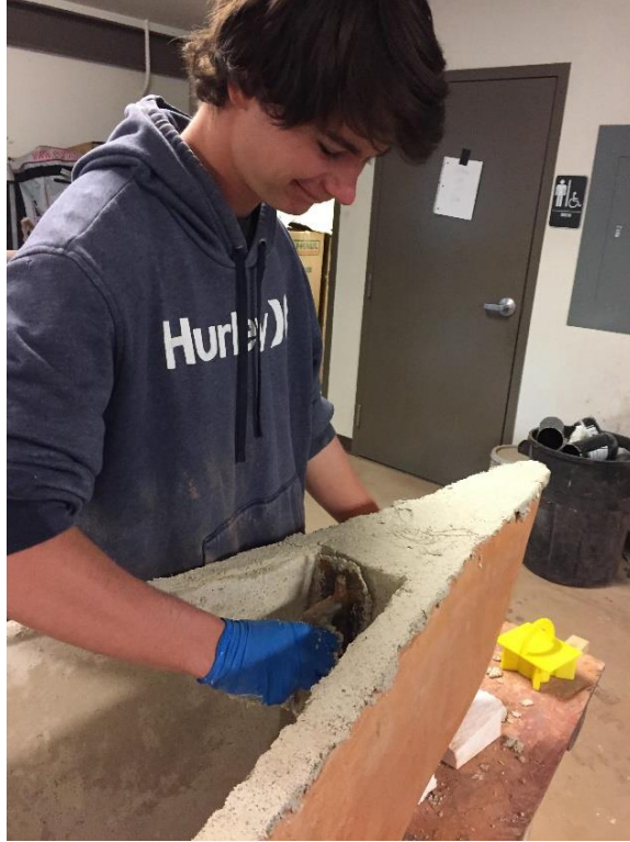
Photo 5. Incasing the Bow/Stern: The floatation in the bow and stern was encased in structural mix #1.
