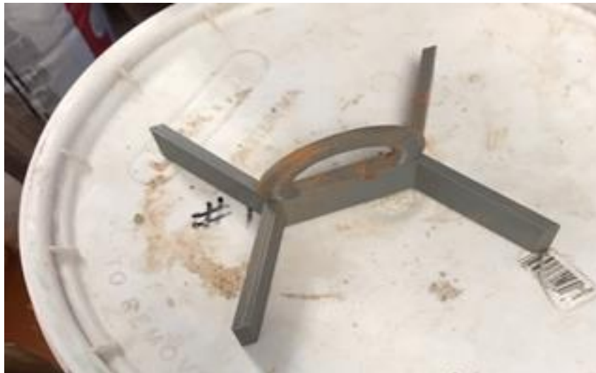
Photo 8. Stencil Imprint: A 3D stencil was printed to create a turtle shell design on the canoe. The ends were aligned when imprinting to develop that hexagonal shape
