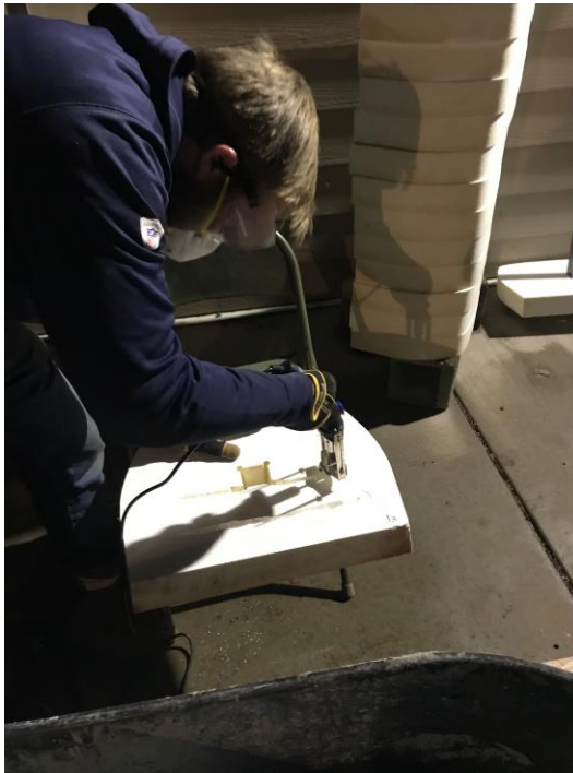
Photo 6. Making Incisions to Mold Cross-Sections: Horizontal slits are made on the face of the cross-section, penetrating through the foam, to aid in the removal of the mold.
