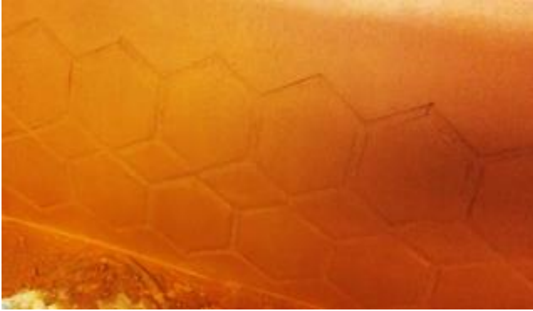
Photo 9. Stencil Pattern: This is the design on the walls of the canoe produced by using the 3D stencil.
