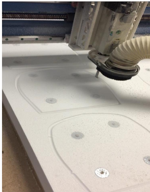
Photo 2. CNC machine Cutting Mold Cross-Sections: Once the hull design was finalized in Prolines and Solidworks, a G-code was made so the CNC router would cut the cross-sections precisely.
