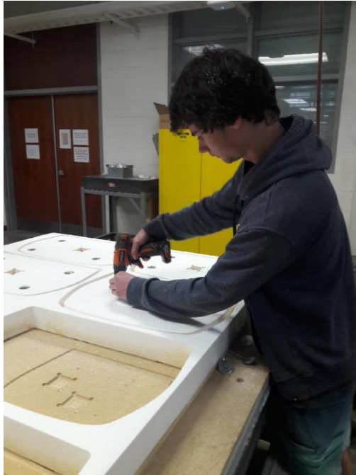
Photo 3. Removing Cross-Section pieces from CNC Machine: After the CNC router completed cutting the first foam block, the next was placed in the machine.
