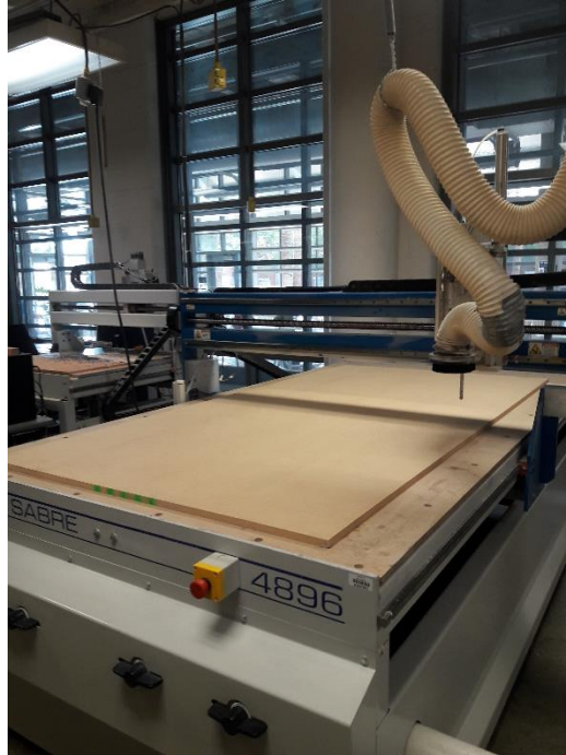
Photo 1. Preparation for Mold Cutting: The construction of the male foam mold was done by using a computer numerical control (CNC) router from a third party. The CNC router cut 4 ft x 8 ft x 3 in. foam blocks into cross-section pieces of the canoe design.
