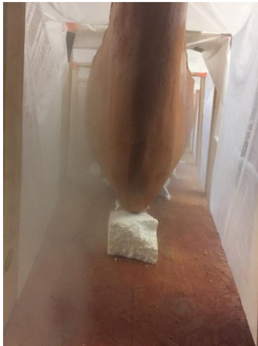
Photo 2. Curing Chamber: The photo above displays the canoe resting on styrofoam slices in the curing chamber. Moisture in the curing chamber was caused by using two humidifiers. The canoe cured for 28 days for it to reach 95% strength.
