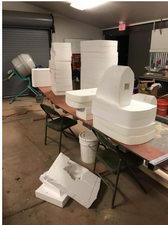
Photo 4. Arranged Pieces of Mold Cross-Section: Once all the pieces were cut, they were transported to the field station (farm). A total of 83 cross-sections were cut from eight foam blocks.
