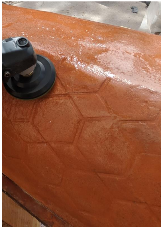
Photo 8. Polishing the Canoe: Polishing the canoe using a wet polisher.
