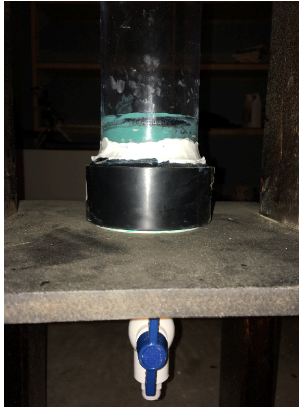
Figure 6: Nozzle Aparatus connected to Column resting on Base
