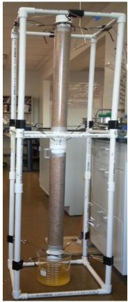
We wanted a minimum of 80% efficiency in this column design. We previously found that 80cm had an efficiency of about 75%. For easy of construction a 120 cm Column height was selected with a 2 cm diameter. Increasing the diameter allowed for an increased loading rate. We hypothesized that this would grant us our desired 80% system efficiency. This system was design with the API system start-up fluid.
