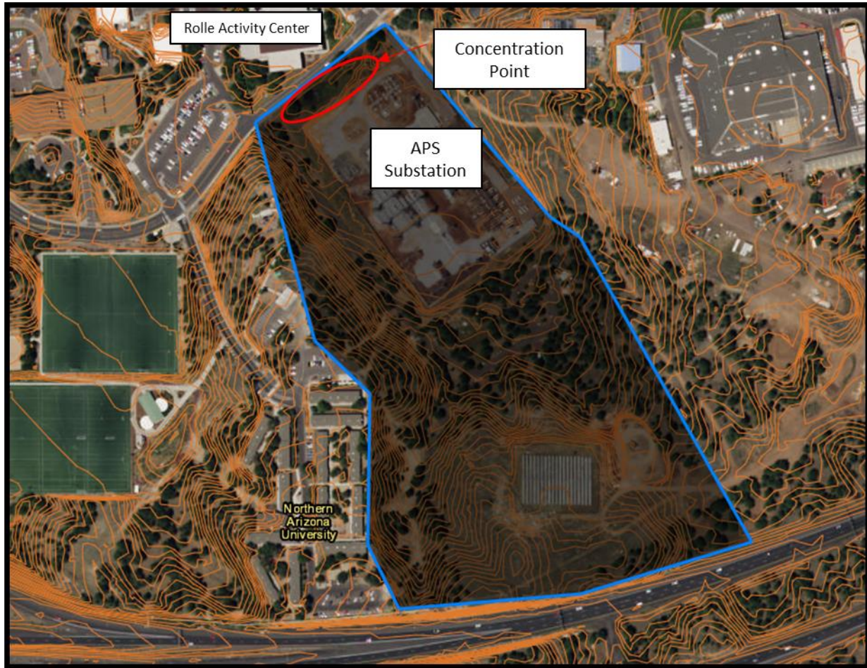
Figure 10. SCS TR-55 CN Method area of basin contributing to the volume of water to the pond in between Pine Knoll Dr. and the APS Substation
