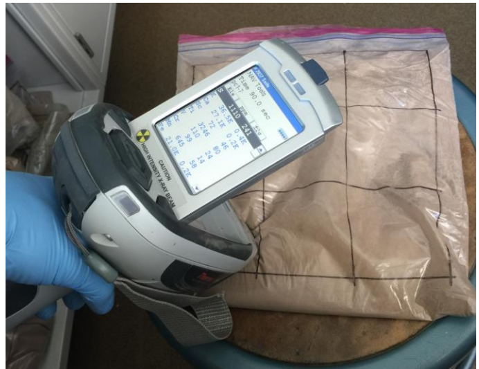
Figure 4.3 - XRF Analysis of a Soil Sample
