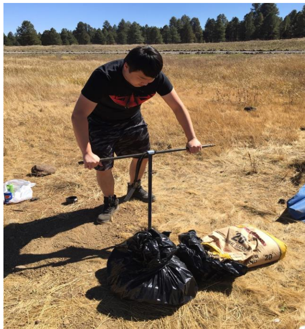
Figure 14: Team member using 6-inches hand auger
