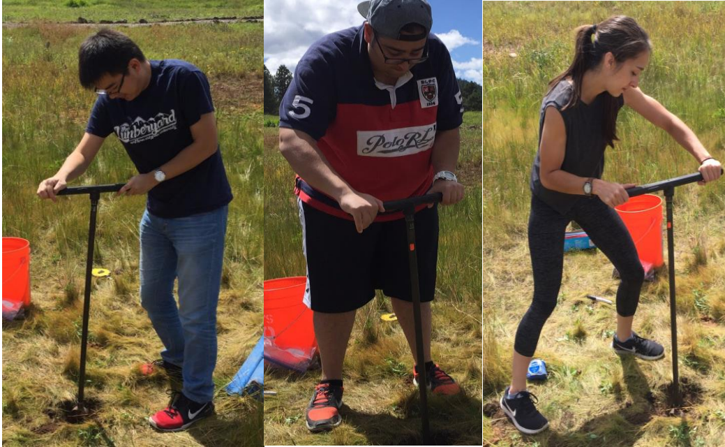
Figure 13: Team members using hand augers for monitoring well hole
