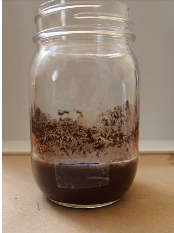
Figure 26: Jar marked after 30-second settling
