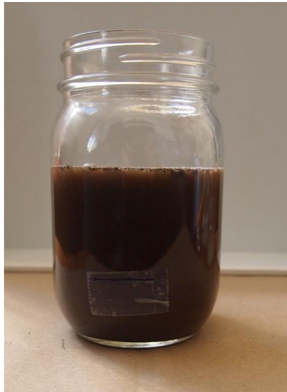
Figure 27: Jar filled with water after 30-second settling period
