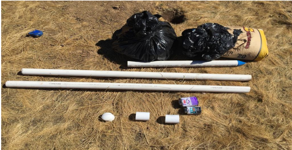
Figure 15: Monitoring well components
