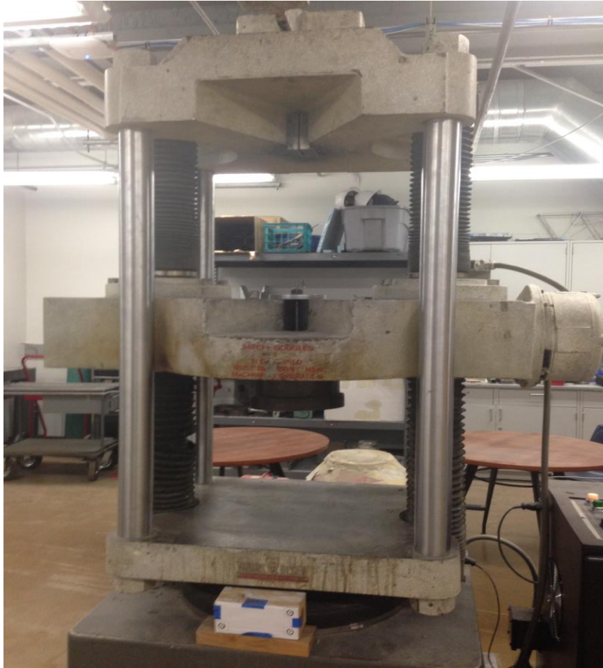
Fig 14 Compression Test Tinius Olsen
