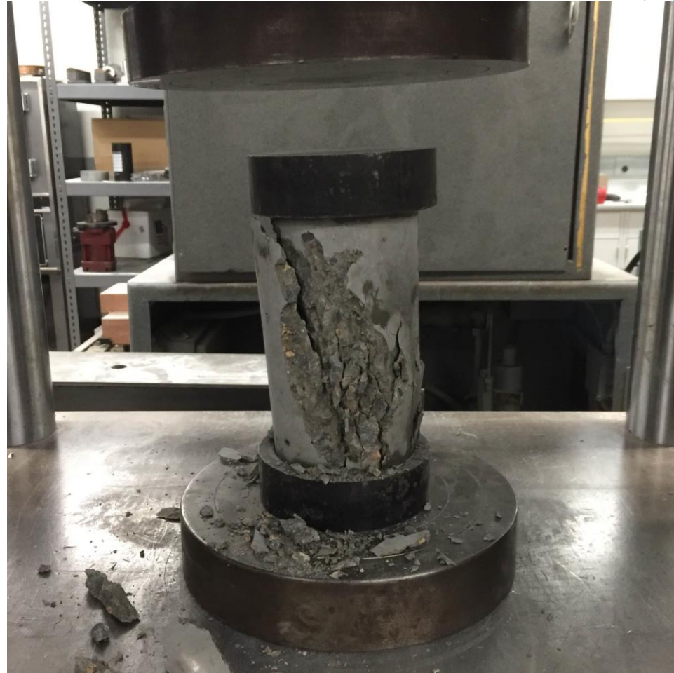
Fig 15 Concrete after Compression Test
