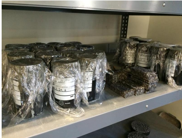
Fig 12 Hardening before removing mold
