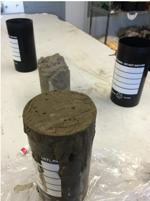
Fig 11 Concrete placed in mold
