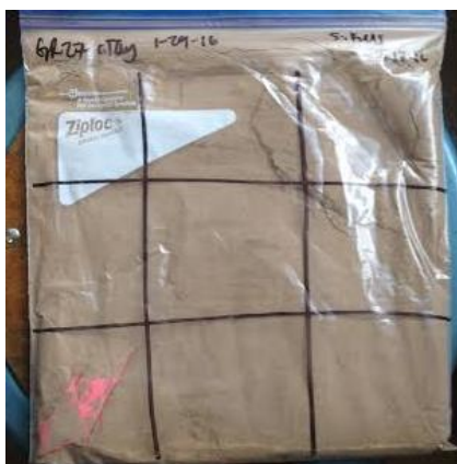
Figure 3.4: 3x3 Grid on sample bags for XRF.
