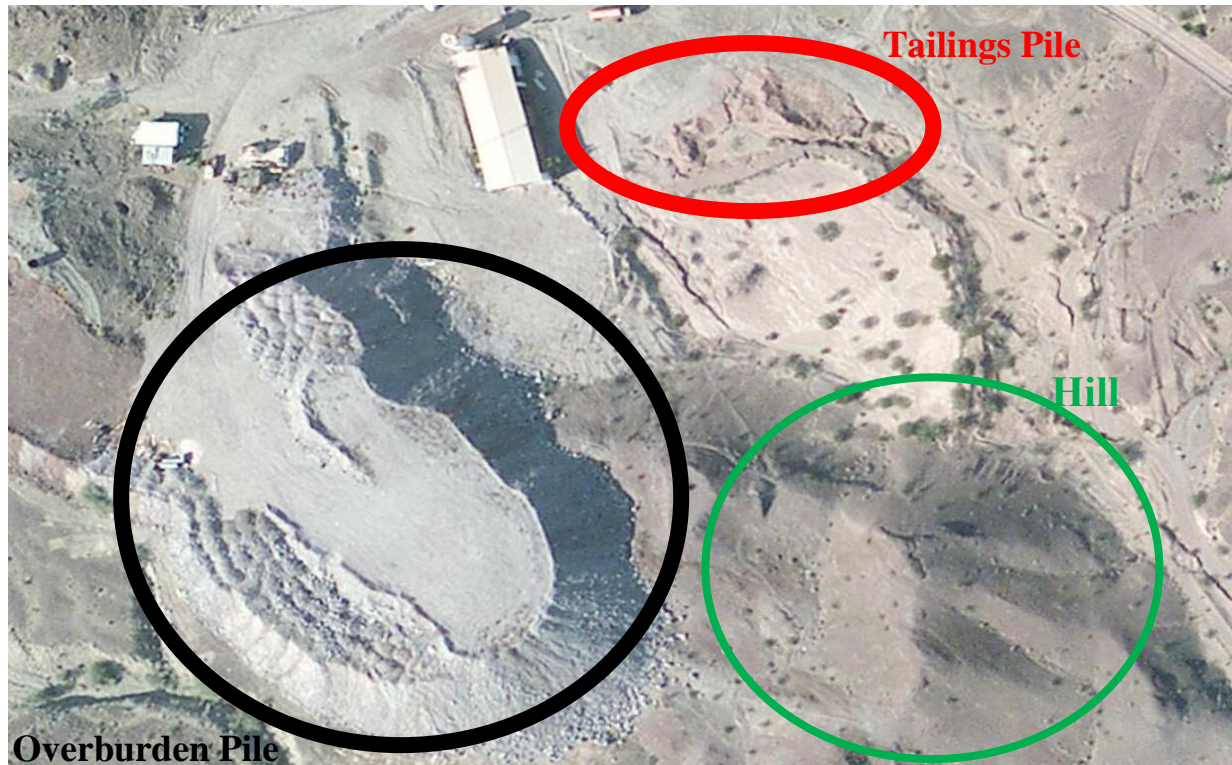
Figure 2.4: GIS image displaying a close up of the actual tailings pile and the overburden pile. Directly north of the overburden pile is Red Cloud Mine.
