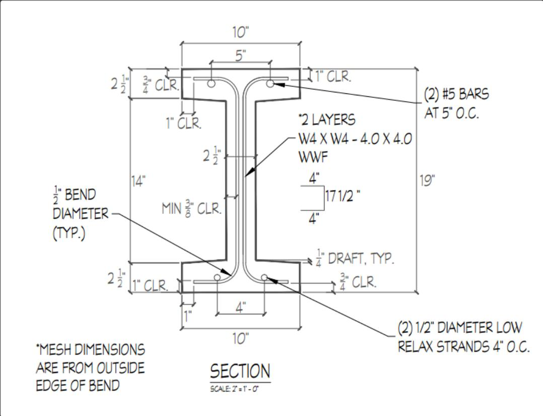
Figure 8: "Final Design Cross Section"
