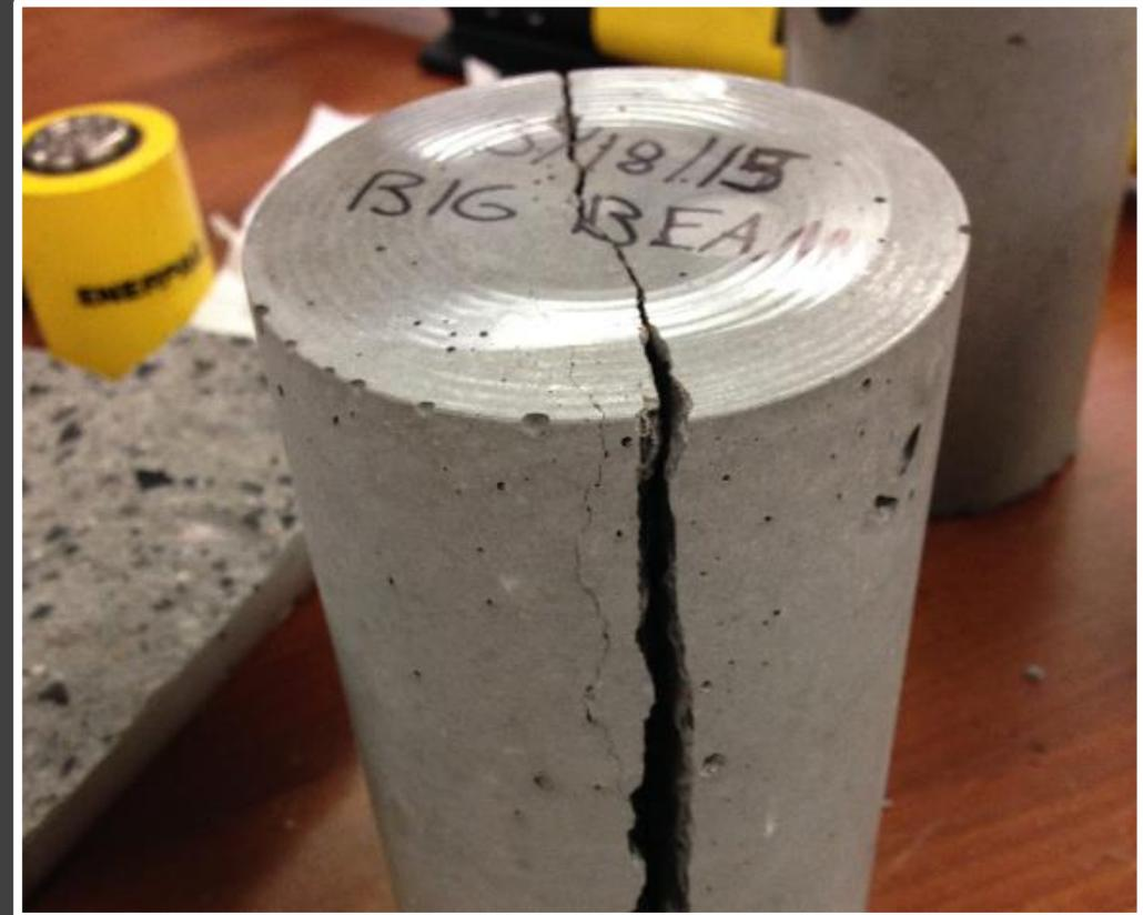
Figure 19: “Broken Cylinder”
