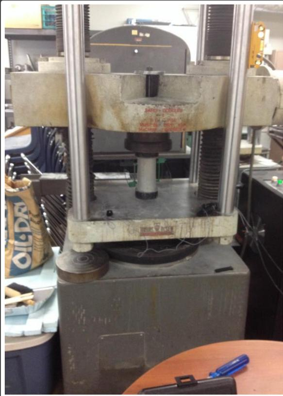
Figure 15: "Axial Compression Test"
