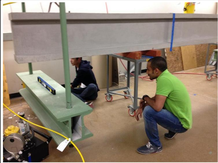
**Figure 12: “Leveling Supports”**
