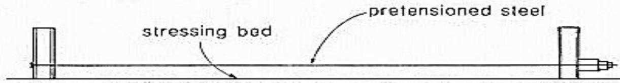
step 1 - tensioning of prestressing steel in stressing bed before casting concrete
