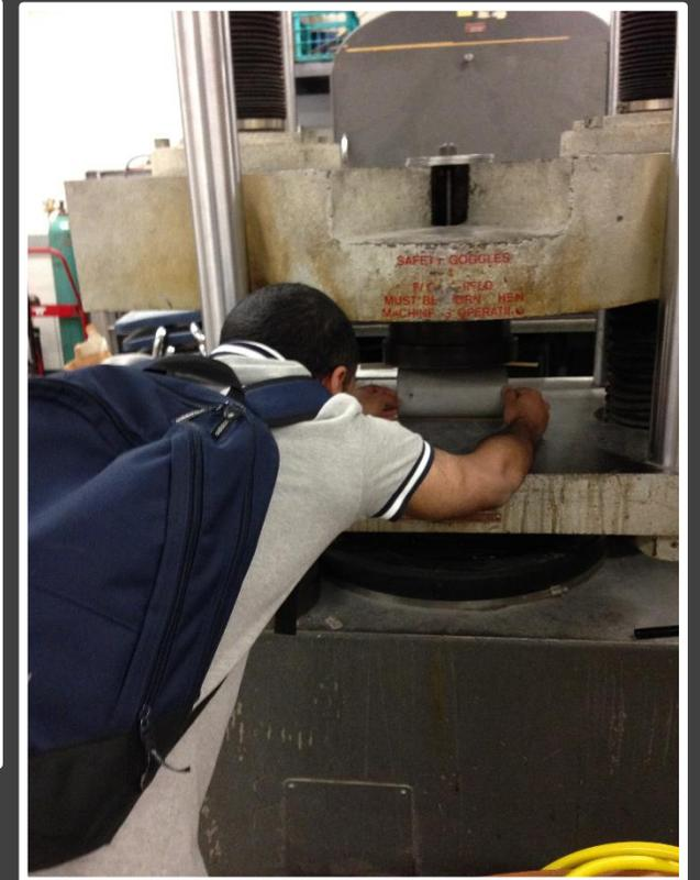
Figure 17: "Split Cylinder Test"
