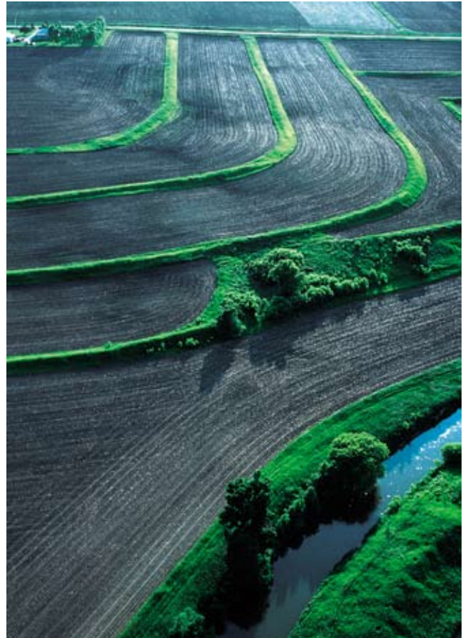
Figure 4-8 Terraces, conservation tillage, and conservation buffers form a system to treat the watershed and protect the stream (Woodbury County in northwestern IA)
