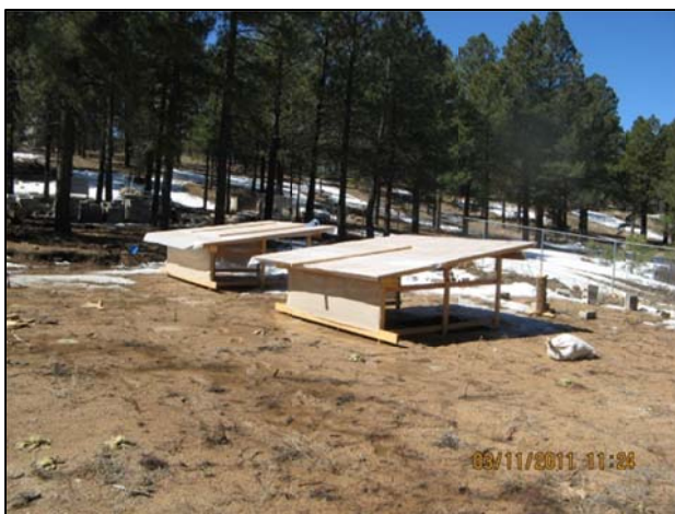
Figure 5: Application of Shade Cloth in an Attempt to Reduce Solar Contamination
