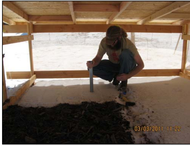
Figure 8: Sampling study plots with constructed sampling tube
