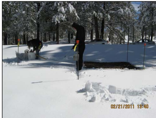
Figure 12: Application of vegetable oil onto snowpack
